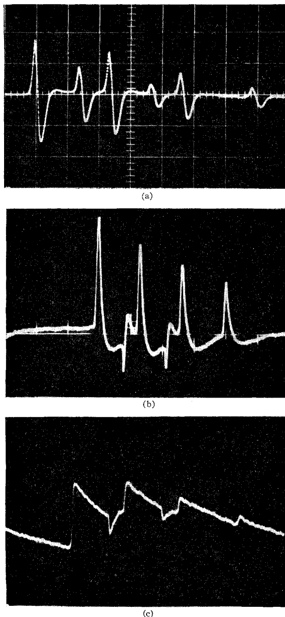
FIG. 8. The Zeeman transitions in polarized Na, showing the effect of the rate at which the magnetic field is swept across the resonance. The magnetic field increases from left to right. The oscilloscope was ac coupled to the photocell, giving a derivative-type line shape. Reading from the left, the second and fourth resonances are the Zeeman transitions in the F=1 hyperfine state. The sweep speed of the magnetic field for the three pictures was 2 sec/div for picture (a), 200 msec/div for picture (b), and 50 msec/div for picture (c). In picture (a) the resonances all have the same general shape of the absorption followed by an RC undershoot (increased absorption caused a bottom to top deflection of the trace). In picture (b) the two Zeeman resonances in the F=1 state have the initial spike of lower absorption followed by increased absorption. In picture (c) the sweep is rapid enough that the light does not pump the system back to equilibrium before the next resonance is reached. In picture (c) the two Zeeman resonances in the F=1 state correspond to lower absorption for the cell and the sweep is rapid enough that the shape of the spike is shown. The pictures (a), (b), and (c) are shown only to explain the effect and were not all taken on the same cell or at the same temperature.
